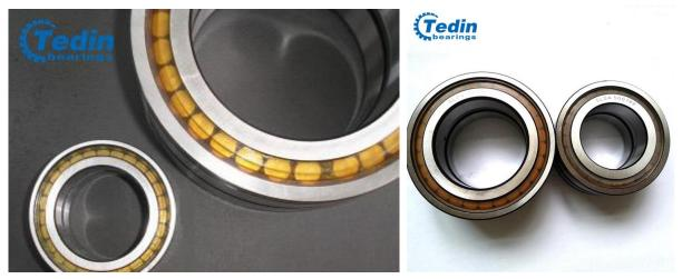
SL04 series full complement cylindrical roller bearings, with sealing rings on both sides and filled with 3# or 2# lithium-based grease. The inner ring is divided into two types: integral cutting type and single processing type, and is fixed by a fixed ring. The outer ring has a central flange, which can be used for axial positioning in two directions. Due to the large distance between the two rows of rollers, the bearing can withstand the overturning moment.
